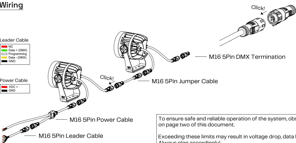
To ensure safe and reliable operation of the system, observe the maximum run lengths on page two of this document.
