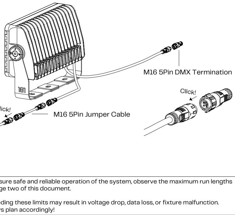
To ensure safe and reliable operation of the system, observe the maximum run lengths on page two of this document.
