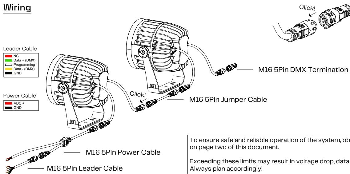
To ensure safe and reliable operation of the system, observe the maximum run lengths on page two of this document.
