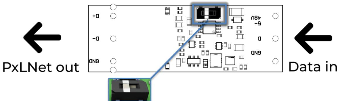
Solder a network or DMX cable to the PxLNet solder pads and connect it to the next PxLNet Transceiver in receiving mode (Rx). It's also possible to have a cable soldered to solder pads [11][12][13] on the underside (as indicated on page 5).
