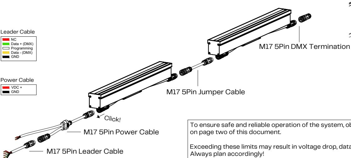
To ensure safe and reliable operation of the system, observe the maximum run lengths on page two of this document.
