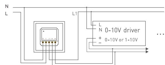
\* An external high-power relay switch is needed when total load current of the dimmer switch is more than 5A or inrush current is more than 50A/0.1S. The damaged dimmer switch resulting from overload current is not recovered by warranty.
