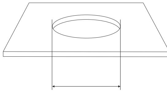
Minimum hole size:  $\phi 48\text{mm}$  (1,89")
