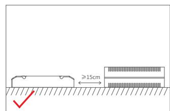
Please do not stack the products. The distance between two products should be  $\geq 15\text{cm}$  so as not to affect heat dissipation and the lifespan of the products.
