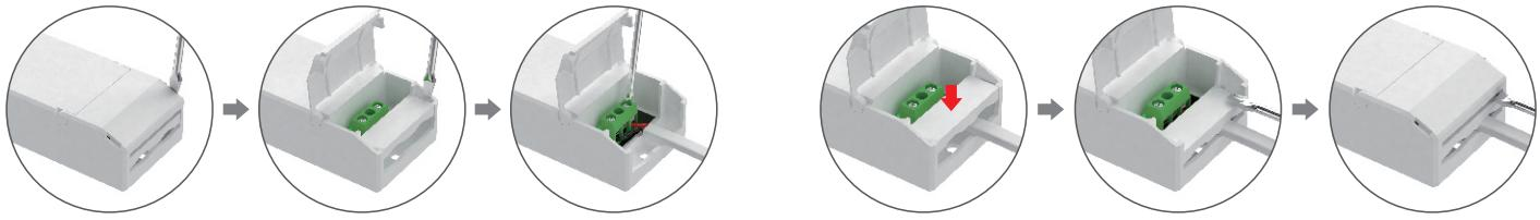
1. Put the head of a screwdriver on the side of the housing to pry up both the protective cover and wire fixing board. Then remove the wire fixing board and connect to the wires as wiring diagram shows.
